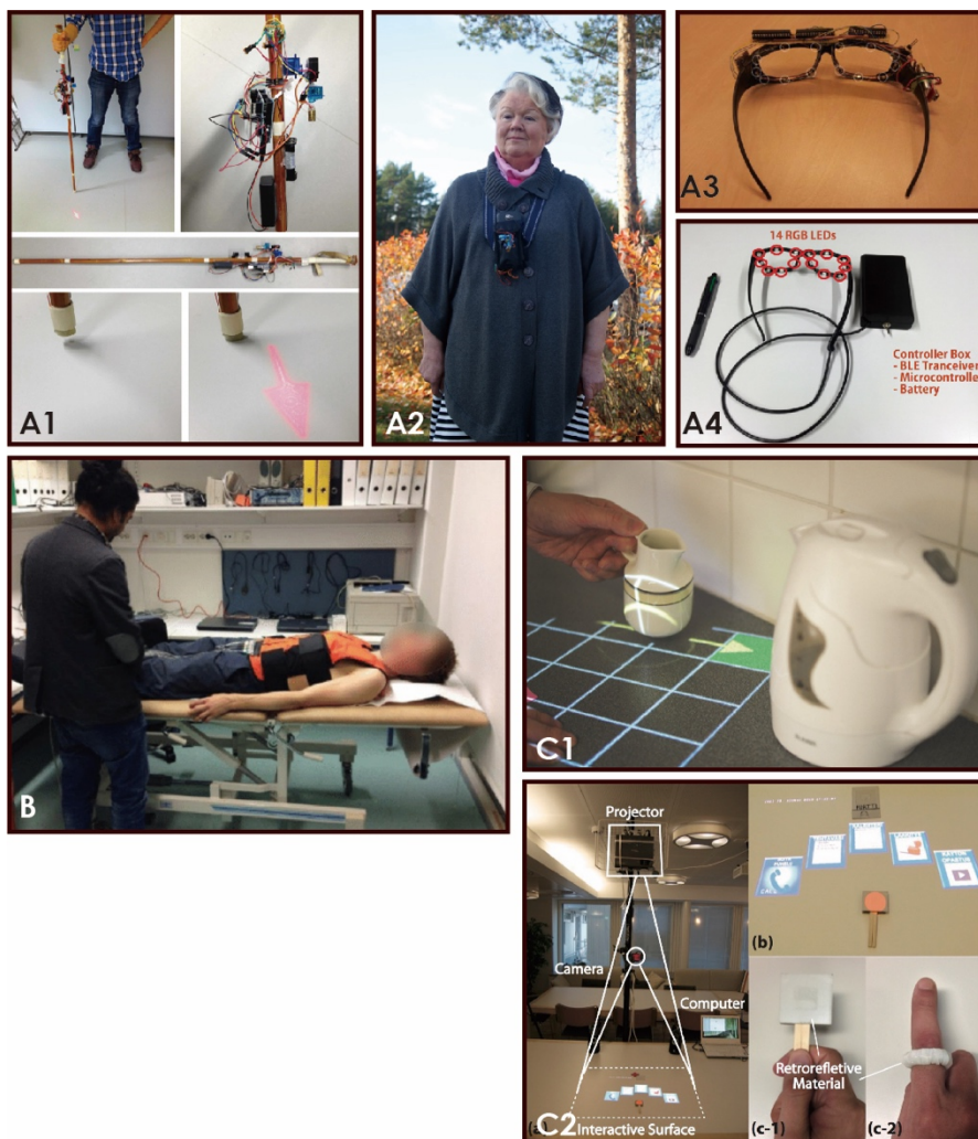
Our system. A1: Cane-type navigation system, A2: Pendant-type navigation system, A3: Smart Megane (first prototype), A4: Smart Megane (light model), B: Sensor vest, C1: Projection remote assistive system, C2: Projection visual input interface.
