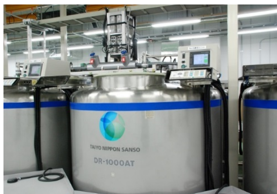
Vapor-Phase Liquid Nitrogen - 180 °C 1,300,000 tubes
