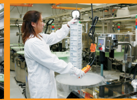
A rack is directly placed in a liquid nitrogen dewar with a handle.
