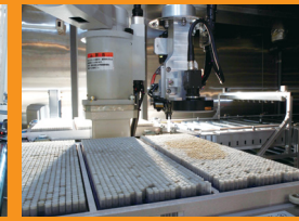
The location of the tube to be picked up is searched for among the tubes on buckets.
