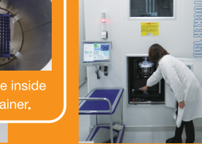
Tubes are stored and delivered within the automatic freezing storage cabinet.
