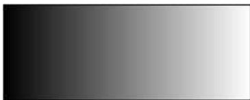
Figure 2-5: The above image has a width of 256 pixels, with a gradation in the brightness spectrum from 0 (completely black) to 255 (completely white). However, the quantitiveness of the extreme ends of this spectrum is lost to the human eye (and print outs).
