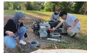
Conducting preliminary measurements of the electromagnetic wave environment to choose equipment installation sites
