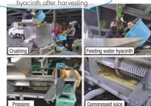
Crushing and pressing water hyacinth after harvesting
