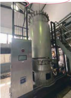
Bench plant where biofuels and chemicals will be produced
