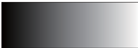
Figure 9 Brightness spectral gradation of an image with 256 pixels in width 25 (Transitions from brightness 0 (black) to brightness 255 (white), one brightness level at a time. The quantitiveness at both ends is not perceivable by human vision (or on printouts).)
